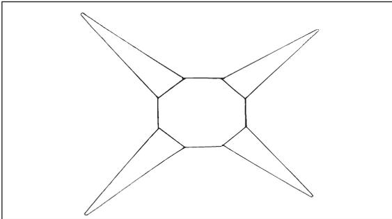
**Step #3** Fold the legs of the dispenser over the coil. Legs overlap each other by 2" so that they can be twisted together to secure the dispenser. If legs are not long enough by themselves, tie wire can be used to secure.
