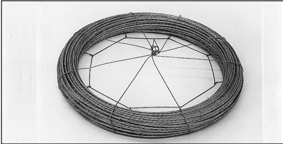
**Step #7** After sufficient strand has been drawn out and cut, the loose end should be placed back in the dispenser. The loose end is now secure and the coil can be moved safely.
