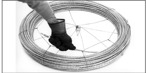
**Step #6** Turn the dispenser over so that the twisted "knot" is down. To pay out the coil, pull out the required length of strand. There is no need to hold the dispenser as the weight of the coil will hold it down.
